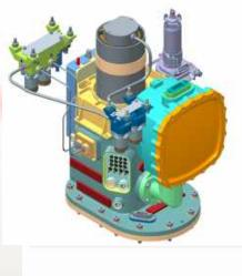
MOMA performs gas chromatograph pyrolysis injections with known gases.
